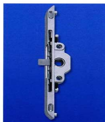
Mill-in gears, 180° with wrong operation safety device are used for tilt-turn sashes; without wrong operation safety device for side hung and tilt sashes(Handles DIRIGENT or ADAGIO-F as shown).
